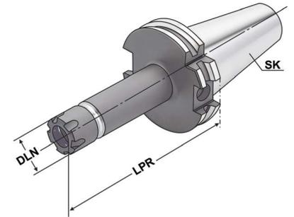
ISO 7388-1    Form AD/AF (AD/B)     $\leq 3\mu\text{m}$     G2.5 25.000 min<sup>-1</sup>    RFID Chip    ISO 15488    13.04
